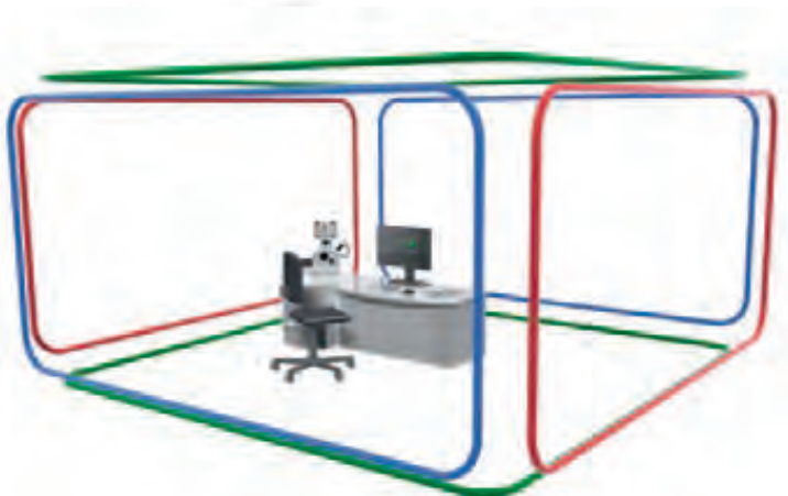
Bilz magnetic field compensation using room coils
