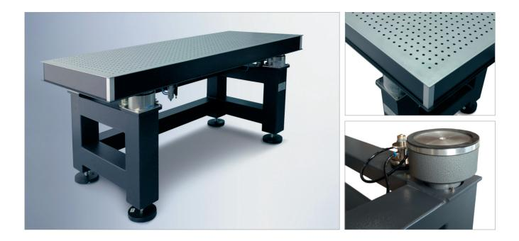
Optical workplaces allow flexible and quick experimental set-ups and offer optimal rigidity and damping at a low weight. The optical table tops have a honeycomb core with high inherent damping and are available with various metal skins with or without threaded holes (raster 25 mm, M6).
